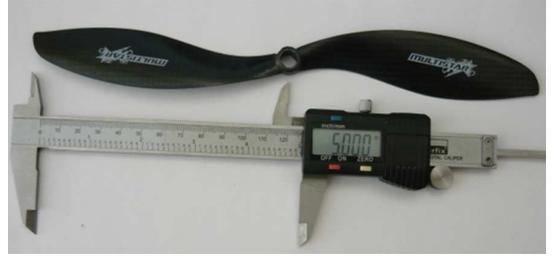
Figure 3. The CFRP propeller used for the measurement.
