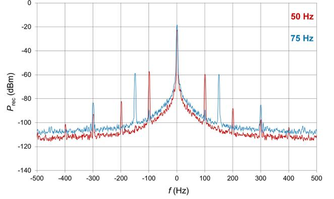
Figure 4. The spectrum of the received signal with two different propeller rotation frequency
