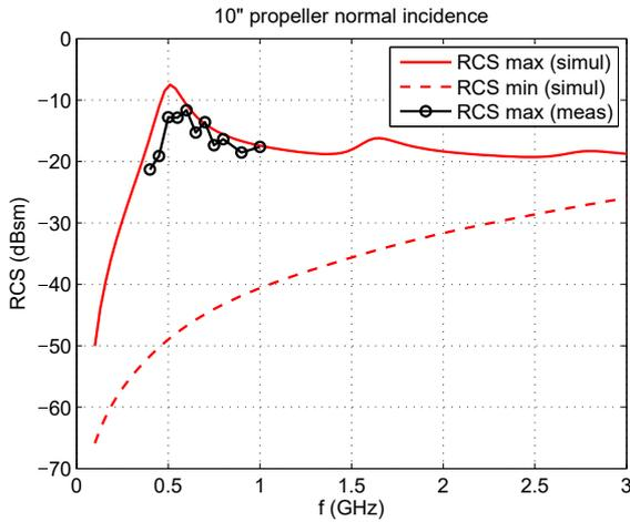
Figure 5. Measured and simulated maximal ( $\alpha = 0^\circ$ ) and minimal ( $\alpha = 90^\circ$ ) RCS values of the propeller, with respect to the excitation frequency. (Unit is decibel-square meter, dBsm.)
