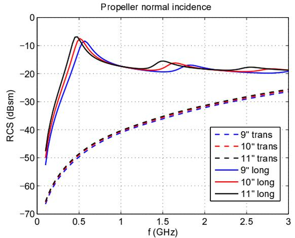
Figure 7. Simulated RCS values of propellers of different lengths  $l$ , for transverse ( $\alpha = 90^\circ$ ) and longitudinal ( $\alpha = 0^\circ$ ) polarization of the incident field. The magnitude and the position of the peak in  $\sigma_{\text{max}}(f)$  moves with  $l$  as expected.
