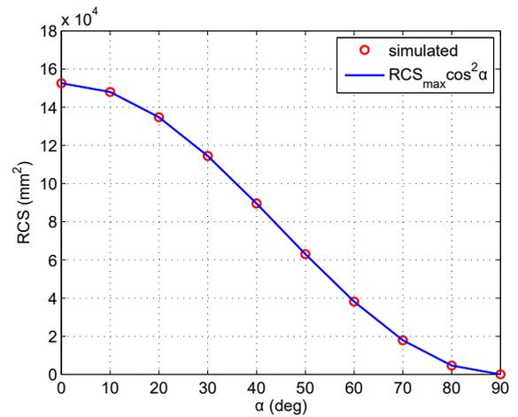
Figure 6. RCS of the propeller at 540 MHz in function of the polarization angle  $\alpha$ . The simulated results perfectly follow the analytic curve proportional to  $\cos^2 \alpha$ .
