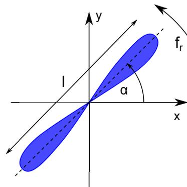
Figure 1. Orientation of the propeller: the rotation plane is the  $xy$  plane, the incident wave propagates to the  $z$  direction and it is polarized in the  $x$  direction.
