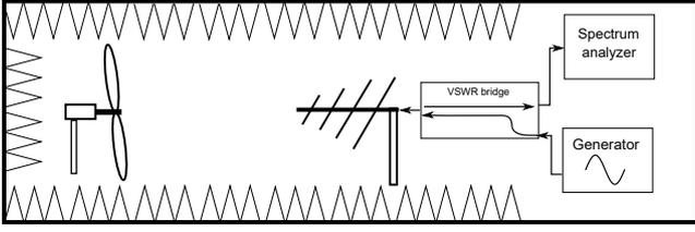
Figure 2. Sketch of the measurement configuration in the anechoic chamber.
